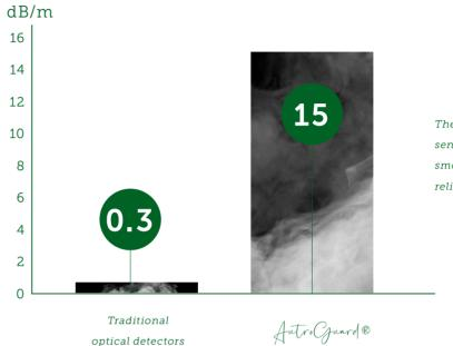
The optical chamber in the AutroGuard® has extreme sensor dynamics, 50 times better than in traditional smoke detectors. This enables a faster and more reliable detection of smoke.
